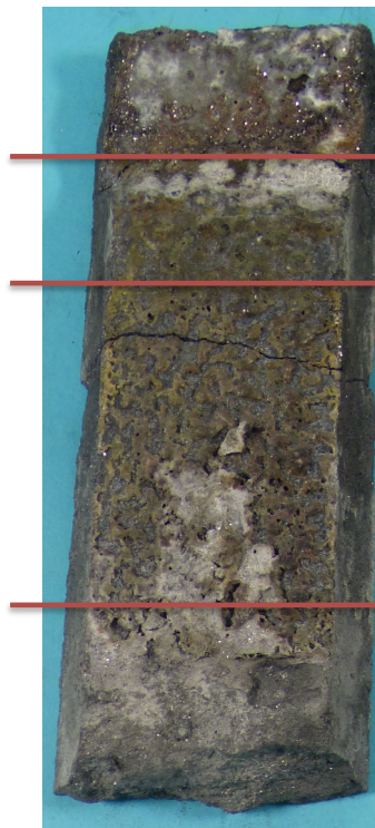
After test with fluoridic slag
