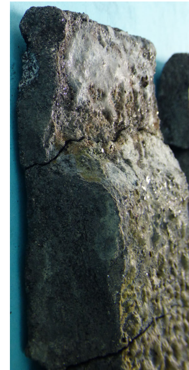
After test with fluoridic slag
